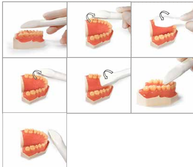
Figure 26: Scan flow for half arch (Single quadrant)
