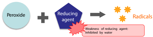
Figure 30. Radical formation explanation in presence of water in conventional resin cement
