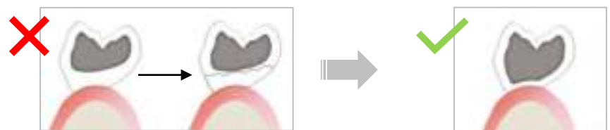
Metal not extended can cause the fracture of the ceramic
