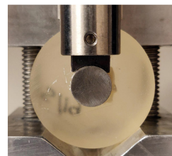
Shear bond test is conducted with 1 mm/min crosshead speed using an Instron model 5866.
