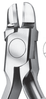
Tweed Arch Bending Plier - .043 Part # GCOA-140 Length: 117mm Maximum Bending Capacity: Rectangular wires up to .022"x.028" Beaks are .043" wide, parallel at .020" opening
