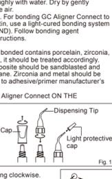
2. Promptly and securely attach dispensing tip to the syringe by turning clockwise.
